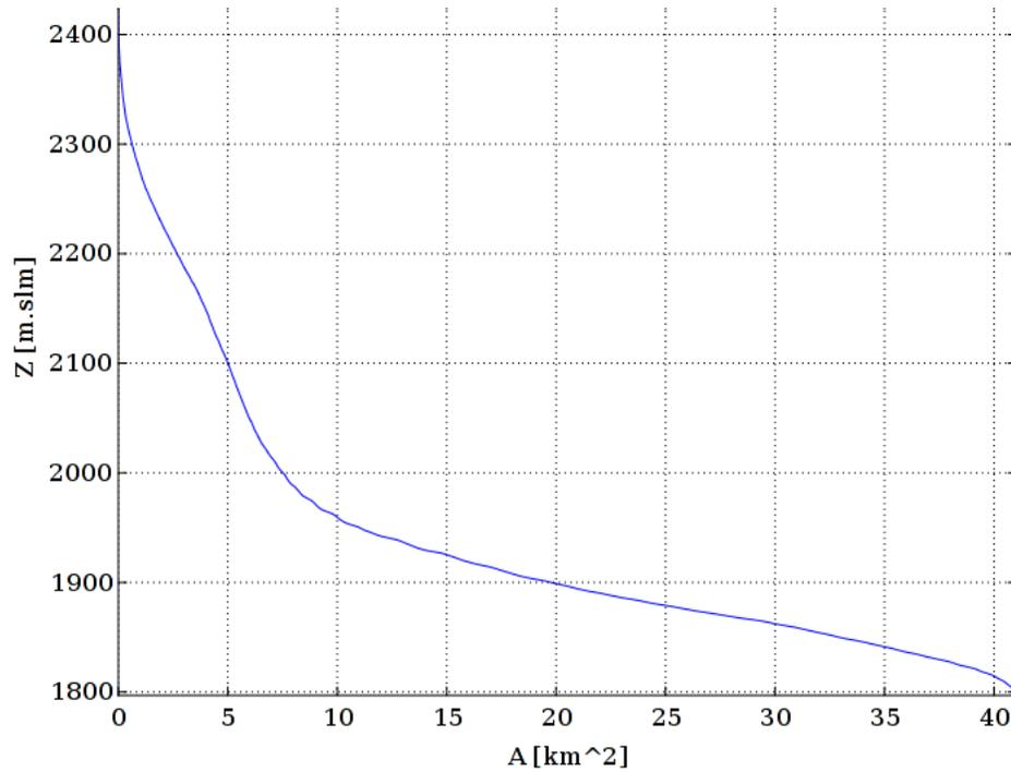
Figure 2.5: Hypsographic curve of the Sheep Creek drainage basin showing the amount of basin area at different elevations. The upper end is comparatively steep but the lower end is much more shallow.
