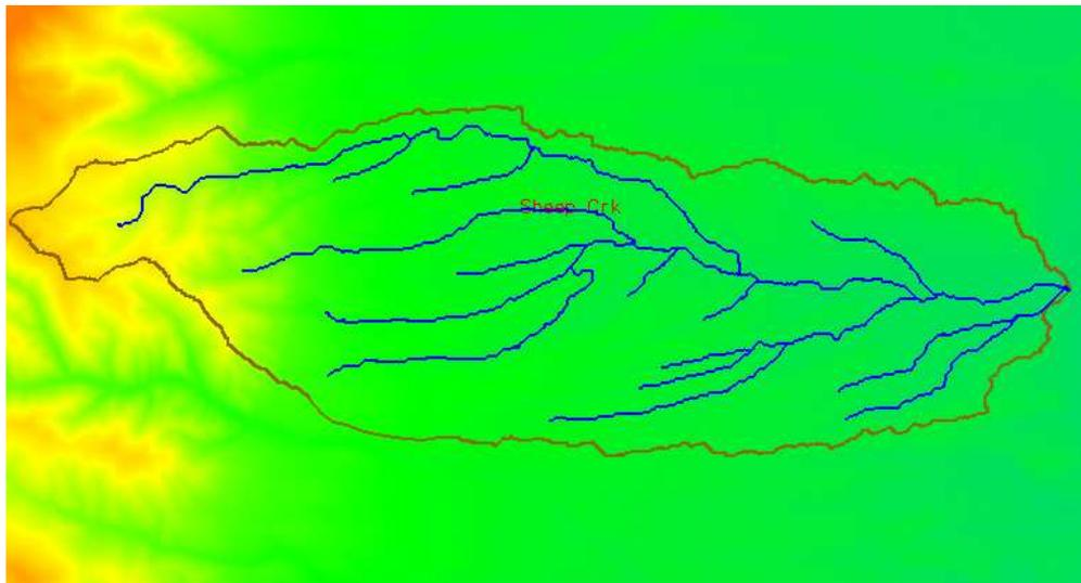
Figure 2.4: Sheep Creek basin and stream network with elevations shown in color.
