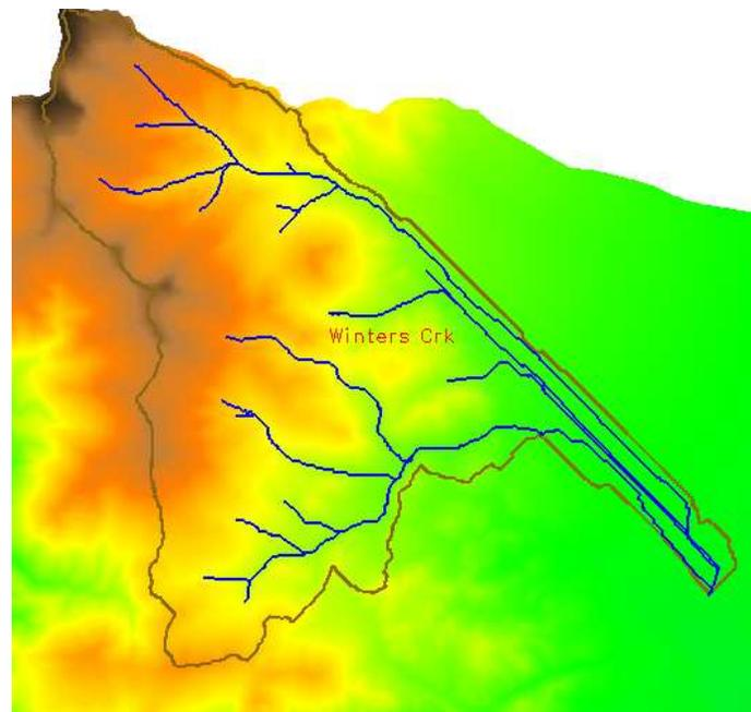
Figure 2.2: Winters Creek basin and stream network with elevations shown in color. The lowest elevation is in green and the colors change to yellow, orange, and brown as elevation increases.
