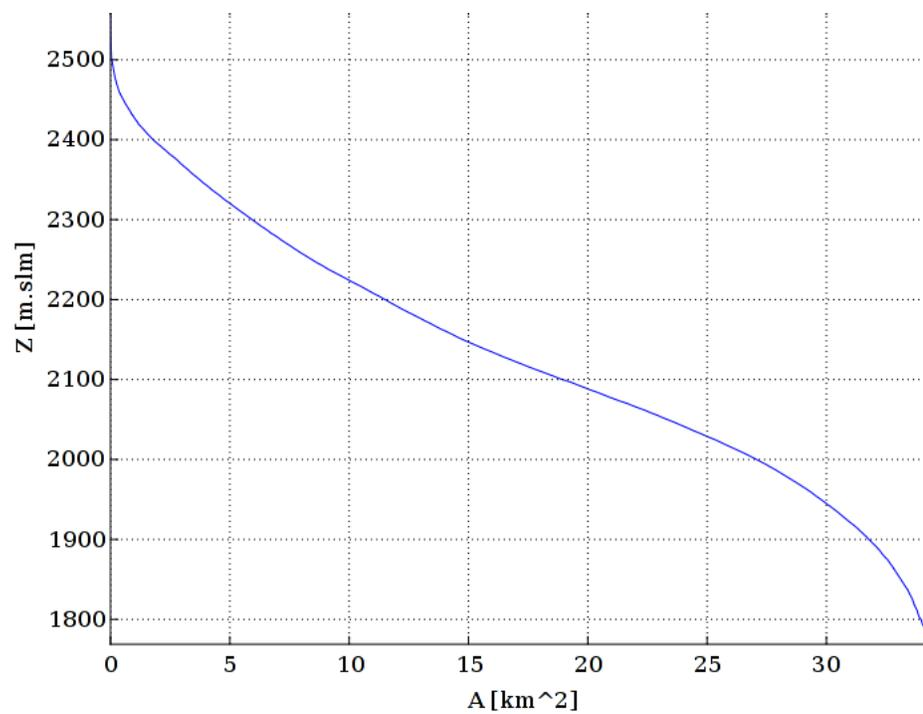
Figure 2.9: Hypsographic plot of basin area at each elevation level for the Jerritt Canyon Creek basin.
