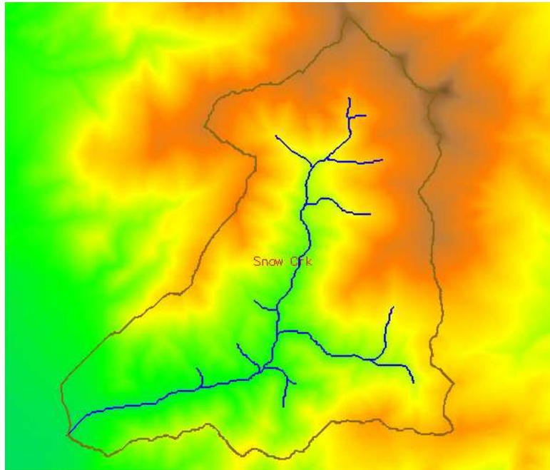
Figure 2.6: Snow Canyon Creek basin and stream network with elevations shown in color.
