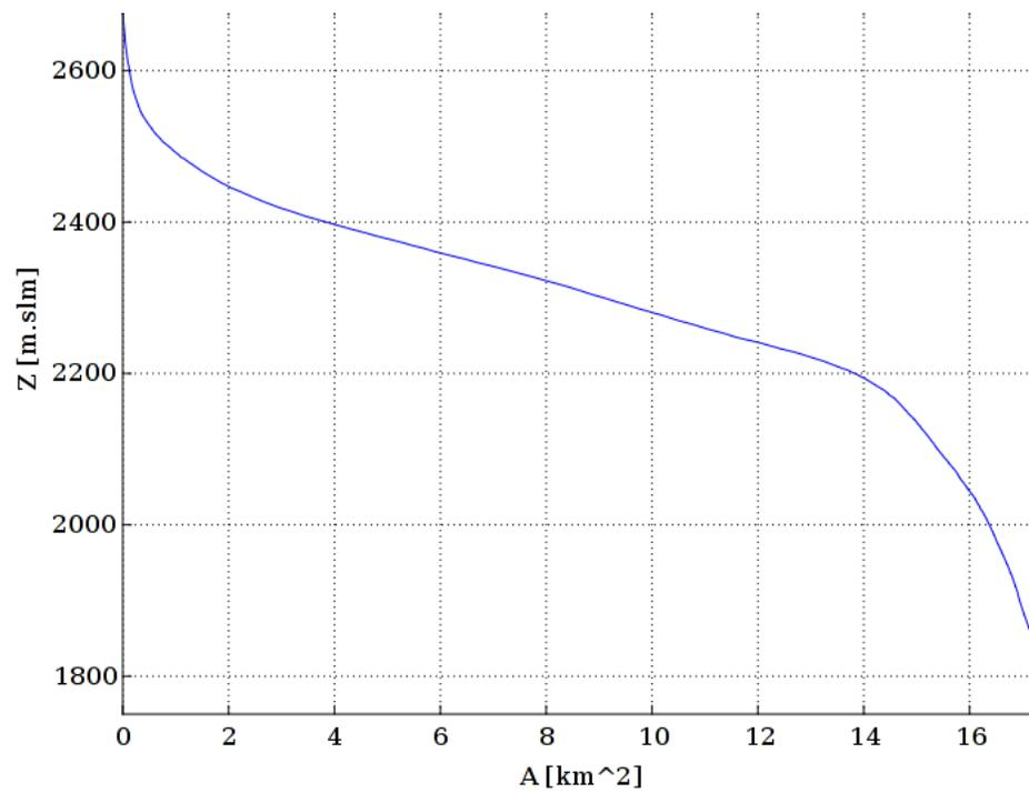
Figure 2.11: Hypsographic curve of Burns Creek basin showing the amount of area at each elevation level.
