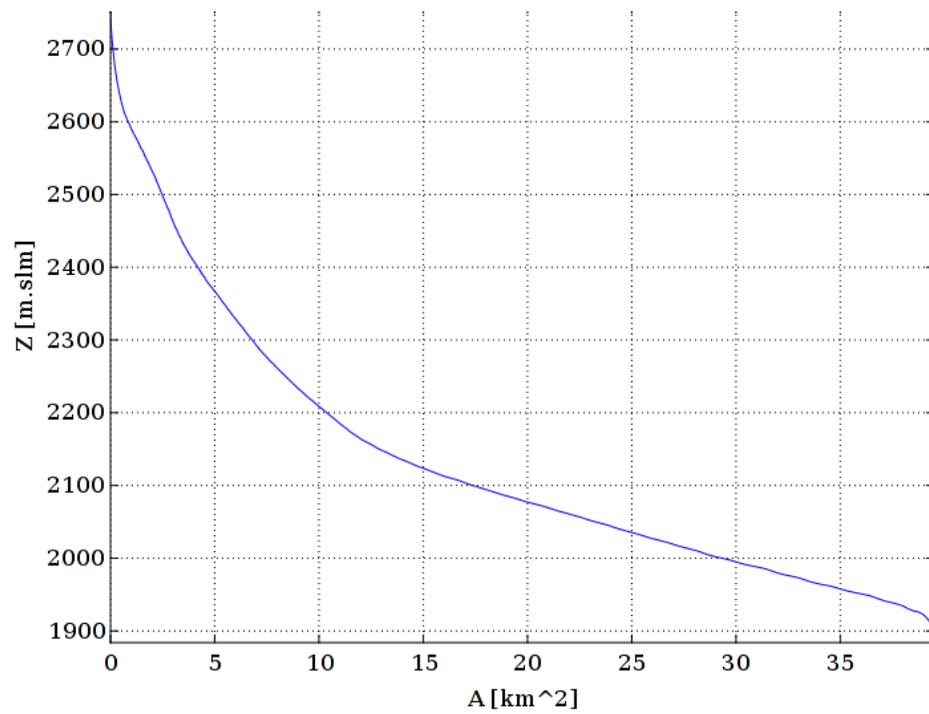
Figure 2.15: Hypsographic curve of the Water Pipe Creek drainage basin showing the distribution of area at each elevation level.
