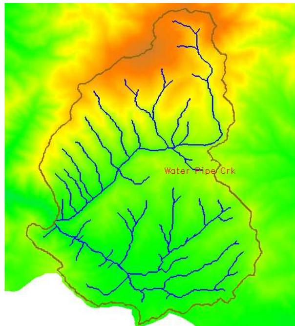
Figure 2.14: Water Pipe Creek basin and stream network with elevations shown in color.
