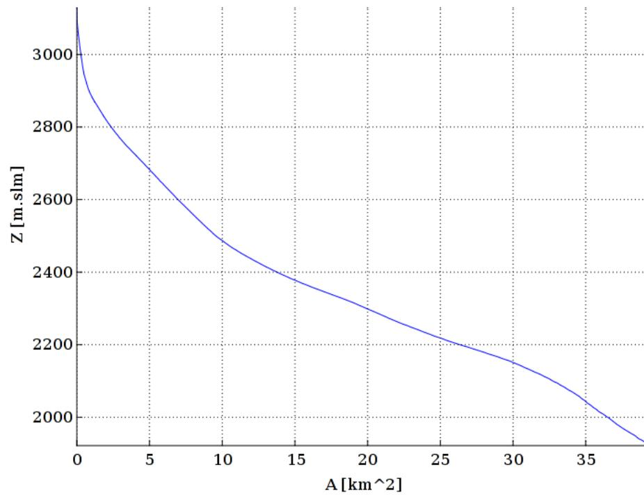
Figure 2.3: Winters Creek hypsographic curve showing the relationship of basin area to elevation. Between 2100–2400 m elevation the basin area decreases linearly from approximately 30 km<sup>2</sup> to 14 km<sup>2</sup> of a total basin area slightly less than 40 km<sup>2</sup>.
