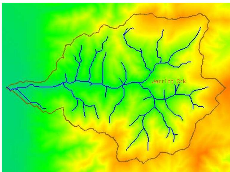
Figure 2.8: Jerritt Canyon Creek drainage basin and stream network with elevations shown in color.
