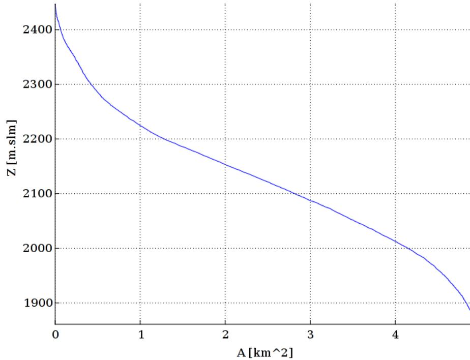
Figure 2.13: Hypsographic plot of Starvation Creek showing the basin area at each elevation level.
