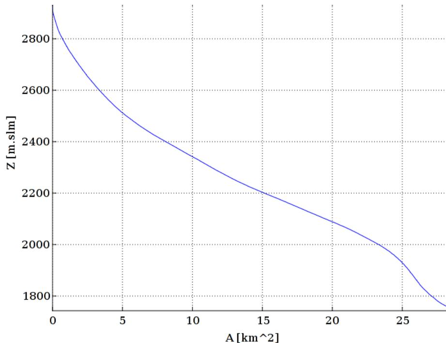
Figure 2.7: Hypsographic curve of the Snow Canyon Creek basin showing the amount of basin area at different elevations.
